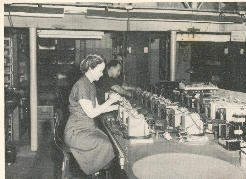
Assembly of power supply for ultrasonic units.
